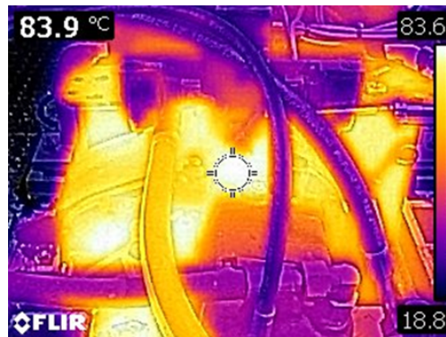
29-3-2019 Total Caprano TD30 - oil temp. 83,9°C
